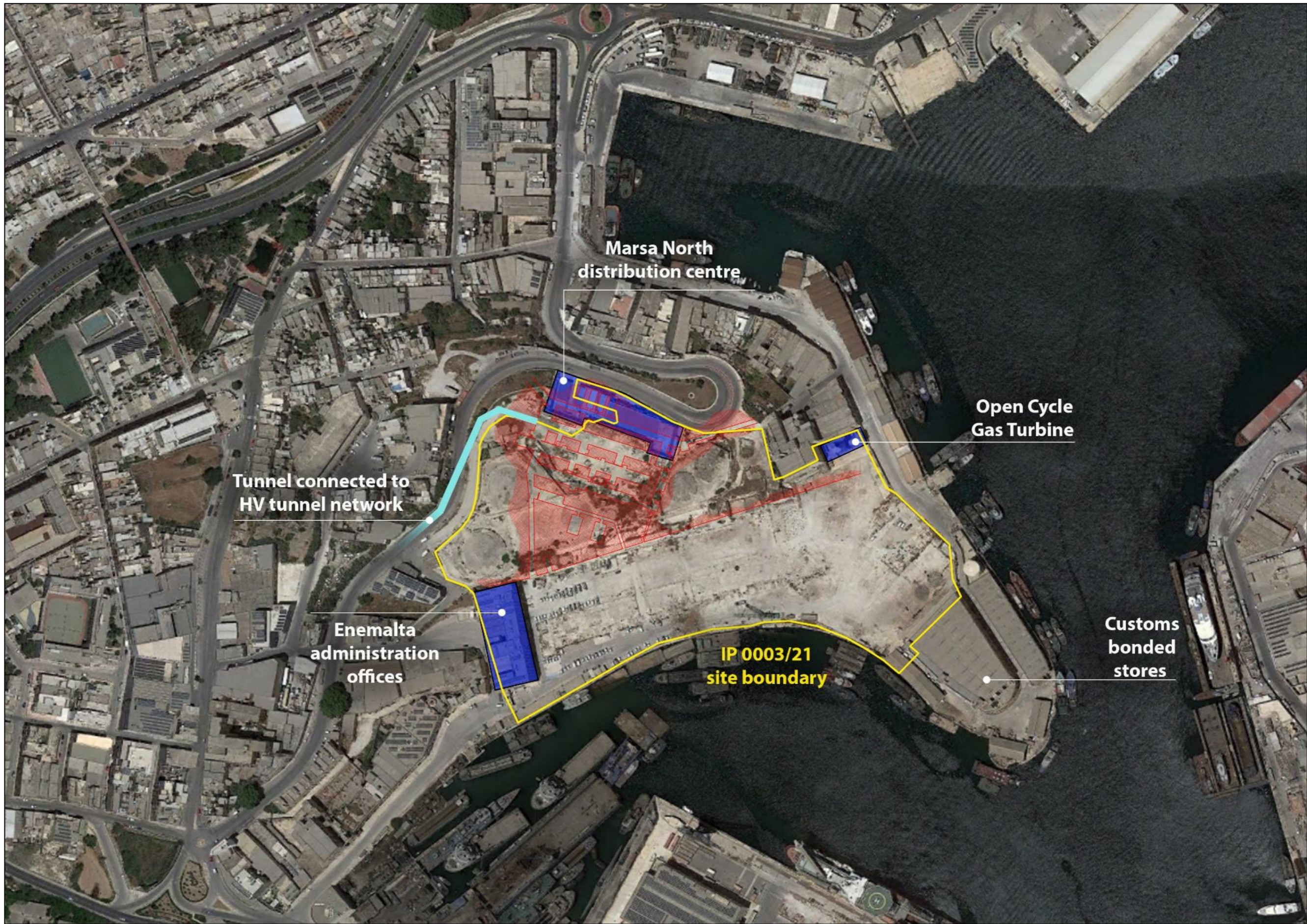
Figure 8: Scheme location A-Station vis-à-vis IP 0003/21 site boundary and other immediate land uses
